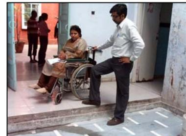
In the Arts Block- Water cooler/taps to be relocated and brought forward (near the edge of the sunken court) to allow everyone to access them with ease
